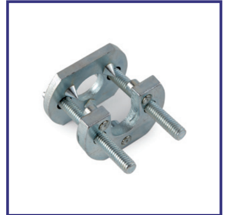
ZDD Plate Crimper tool locks the stub cap into the pot by three crimp indentations. This is a low cost tool with a life of approximately 100 operations. Available in 20mm, 25mm, 32mm & 40mm sizes.
